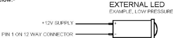
To drive control relays, you need to select a relays of more than 120 Ohms coil resistance (so it draws less than 100mA). You will also **MUST** use a protection diode to clamp the high voltage back EMF resulting from the relay coil when it is de-energised. Please follow the diagram below:-Relay Suggestion:-
